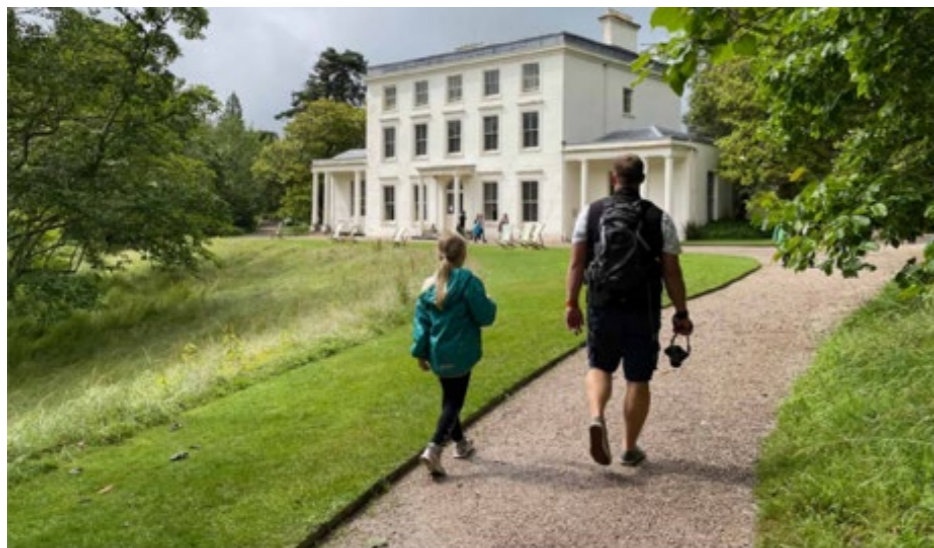
Fig.144 Sinuous paths will allow visitors to meander through the landscape, defined by self-binding aggregate and concealed steel edging.
